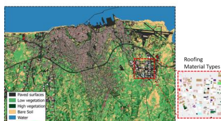
Roofing material classification using spectral library from fused Sentinel-2 and WorldView-2 imagery in Heraklion.
