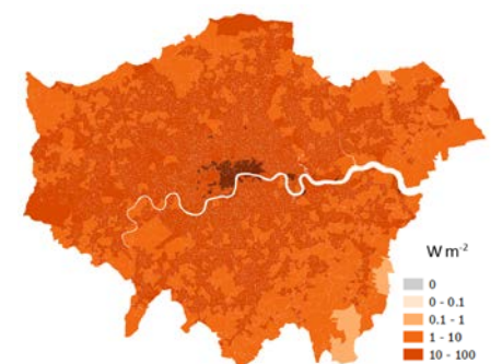
Total anthropogenic heat flux in Greater London (October 2, 2015). Time step used was 10:30-11:00 UTC to coincide with the satellite overpass.
