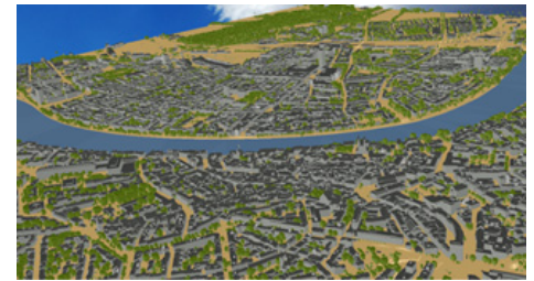
3D view of Basel generated using DART. The Discrete Anisotropic Radiative Transfer (DART) model is a physically based 3D model simulating the Earth-atmosphere radiation interaction from visible to thermal infrared wavelengths.
