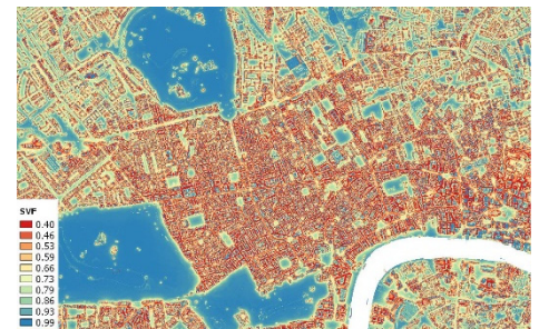
Sky-view factor for a part of London. The sky-view factor is the fraction of sky visible from the ground level. Varies with height and spacing of buildings and trees and affect the surface radiation heating/cooling.
