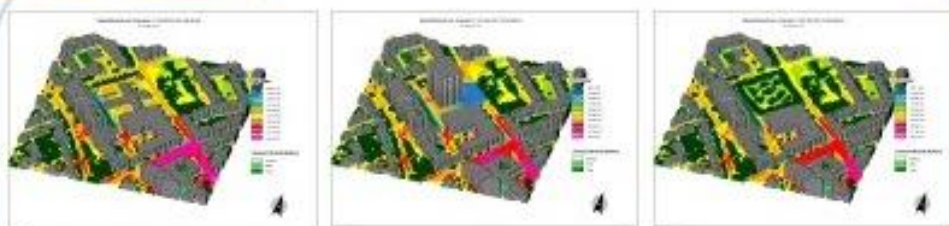
Fig. 4-6: Simulated PMV maps above the ground at 15:00 21.06.2015 for scenarios prison (left), skyscraper and park (right) with buildings (grey) and vegetation (green) as a 3D environment.
