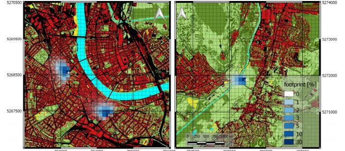
Fig. 4. Weighted footprints for 30 AUG 2015 satellite overpass (11:00 UTC+1). Left: Urban flux towers BKLI and BAES. Right: Rural/suburban flux tower BLER. Reference system is UTM 32N.
