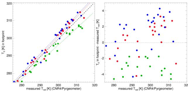
Fig. 6. Left: As fig. 5 but for surface temperature  $T_{rad}$  (x-axis) against satellite derived surface temperature  $T_s$  (y-axis) Right: Same as left panel, but for the differences  $T_s - T_{rad}$
