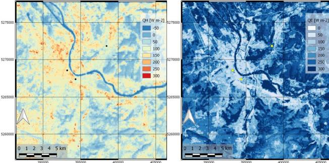
Fig. 2. Modeled sensible heat flux (left) and latent heat flux (right) for Basel during Landsat 8 overpass on 30 AUG 2015. Black and yellow points mark flux towers BKLI, BAES and BLER (from left to right).
