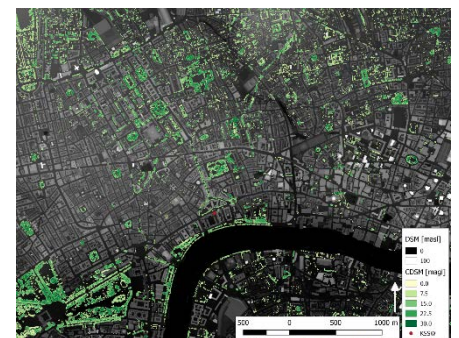
A building and ground DSM overlaid with a vegetation canopy DSM (CDSM) over the central parts of London. The pixel resolution is 1 m x 1 m. Location of Eddy Covariance tower (KSSW) is included. The surface models are derived from LiDAR data.
