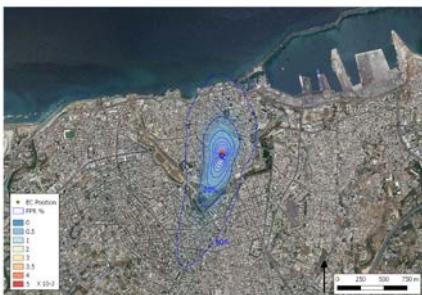
Long-term turbulent heat flux source area (November 2016 - January 2017) of the Heraklion Eddy Covariance measurements.
