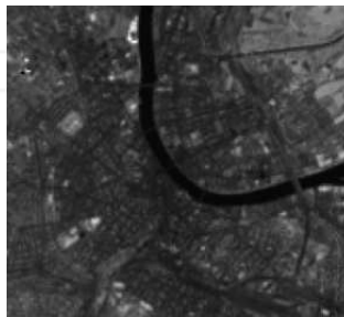
Figure 9. Landsat-8 atmospherically corrected image for an NIR band (864.6 nm) over the city of Basel, acquired on the 24th April, 2015.
