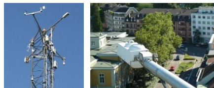
Top of BKLI flux tower with instrumentation for turbulent fluxes of momentum, sensible and latent heat and CO 2 , radiation, wind and wind direction (Right). Close up to the BKLI radiation sensor (Left).
