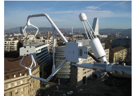
BAES Instrumentation: Campbell Scientific CSAT Sonic (left) and LiCOR-7500 IRGA (Infrared Gas Analyzer).
