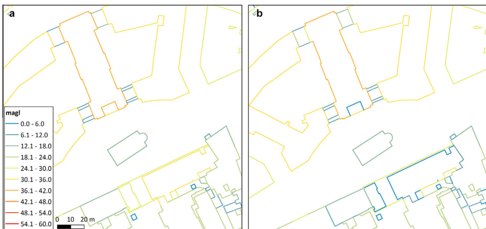
Fig. A1. Wall heights represented as left; height above ground level and right; height difference between ground or adjacent building.
